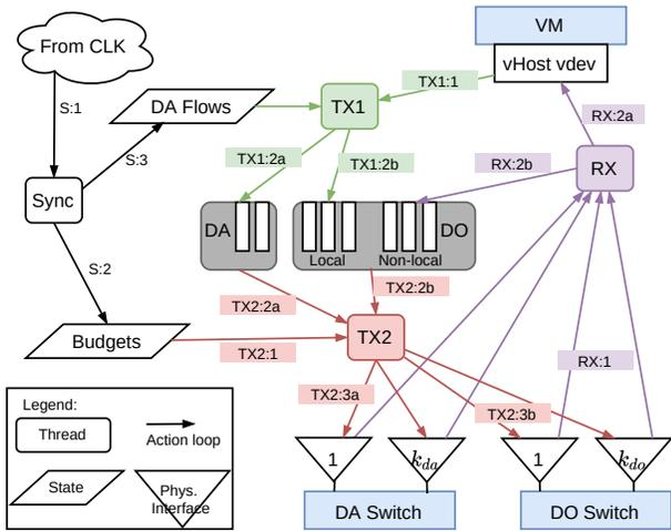
Figure 2: Overview of the DPDK-based ToR emulation.
