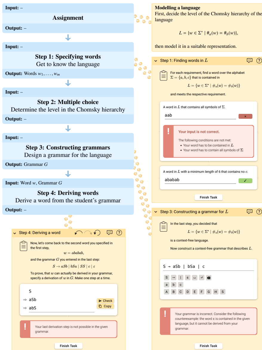
Figure 4: An exercise for constructing a representation of a formal language. As preparatory step, students explore the formal language by identifying some elements and deciding its level in the Chomsky hierarchy. For constructing a representation of a context-free languages LRIS supports context-free grammars and push-down automata; for regular languages, it supports (non-)deterministic finite state automata and regular expressions.
