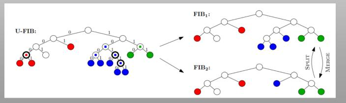
Nodes with square inside: mergeable. Nodes with bold border: suppressed for FIB1.
