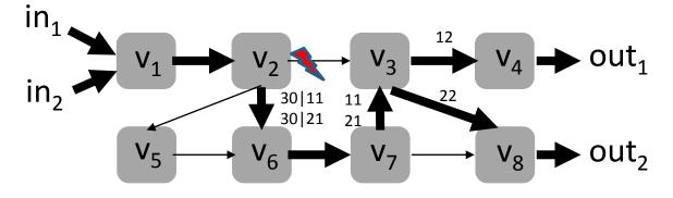
One failure: push 30: route around  $(v_2, v_3)$
