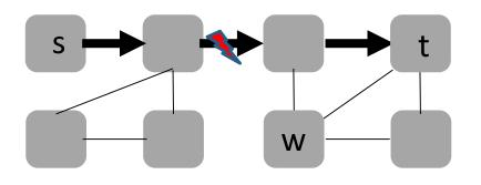
Upon failure: can **push** an intermediate (remote) destination (waypoint), or an adjacent **link** (force)
