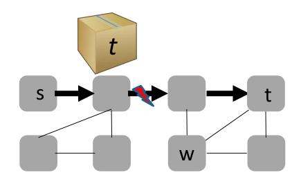
Upon failure: can **push** an intermediate (remote) destination (waypoint), or an adjacent **link** (force)
