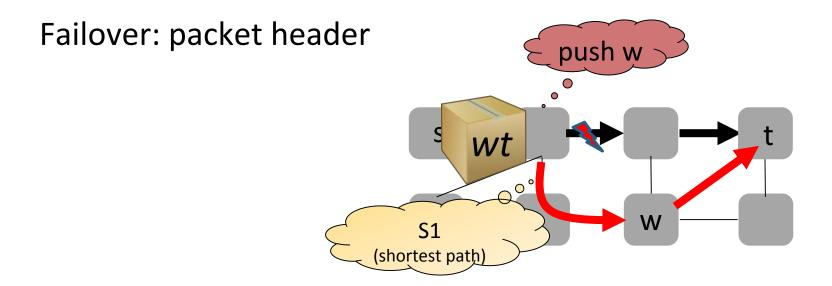
Upon failure: can **push** an intermediate (remote) destination (waypoint), or an adjacent **link** (force)
