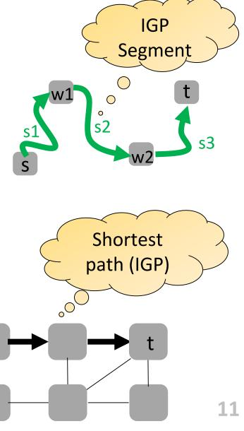
Upon failure: can **push** an intermediate (remote) destination (waypoint), or an adjacent **link** (force)
