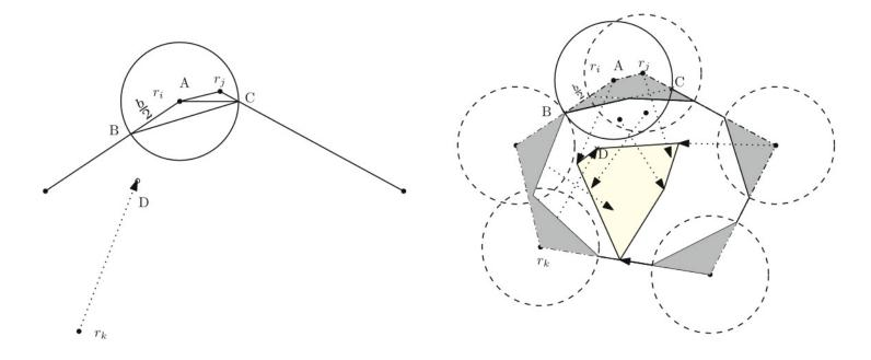
In the figure (right) the shadowed area is the decrement considered for each corner and the central convex hull inside solid lines is the new convex hull after every robot moves.
