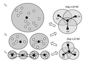
Fig. 2. Decomp constructs independent sets of larger and larger range (left) with fewer active nodes (dark). Knowledge is transferred via the neighborhood covers (right).
