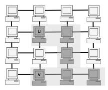
Fig. 1. After hitting the event component (shaded), the event nodes S (dark) need to determine the component size (here: 6). In the onduty model, node u may reach node v in two hops (via a non-event node); in the off-duty model, these two nodes are at distance four.
