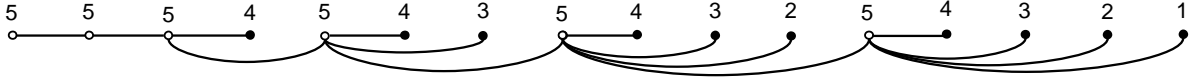
Figure 8. The interference of the exponential node chain—shown in a logarithmic scale—is bounded by O(\sqrt{n}) by the topology control algorithm \mathcal{A}_{exp} . Only hubs (hollow points) interfere with the leftmost node. For clarity of representation edges are depicted as arcs.
